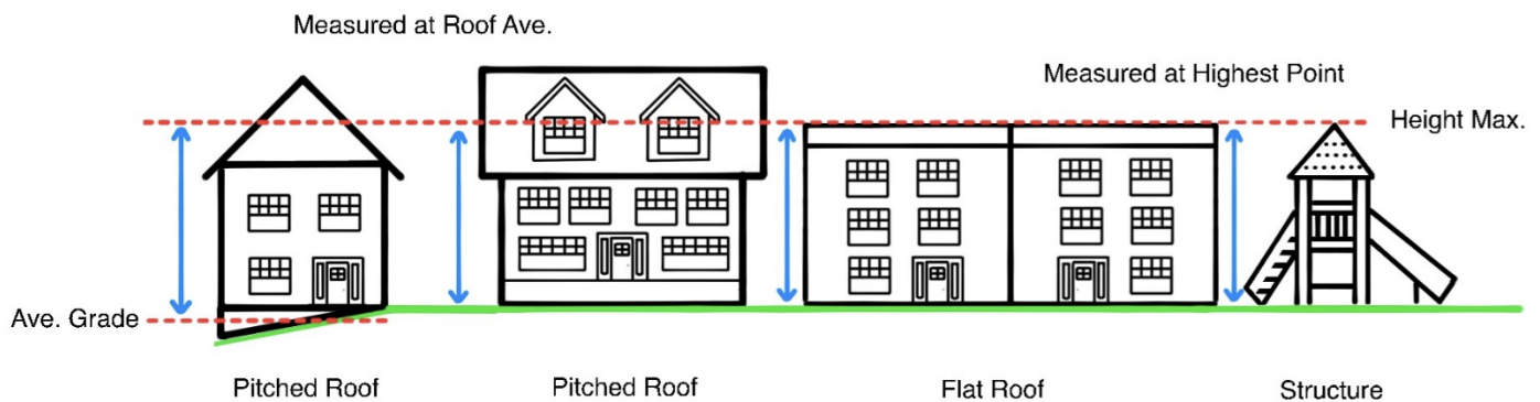
Figure 3-1 Building and Structure Measurements
